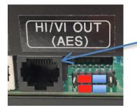
AES Pair 4 / Channels 7/8 are routed directly to the "HIVI OUT" RJ45 connector.
