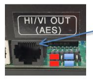
AES Pair 8 / Channels 15/16 are routed directly to the "HIVI OUT" RJ45 connector.
