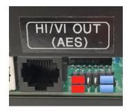
AES Pair 8 / Channels 15/16 are converted to analog signals, and routed to the "Analog HI/VI" pluggable connector.
