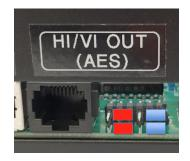
AES Pair 4 / Channels 7/8 are converted to analog signals, and routed to the "Analog HI/VI" pluggable connector.
